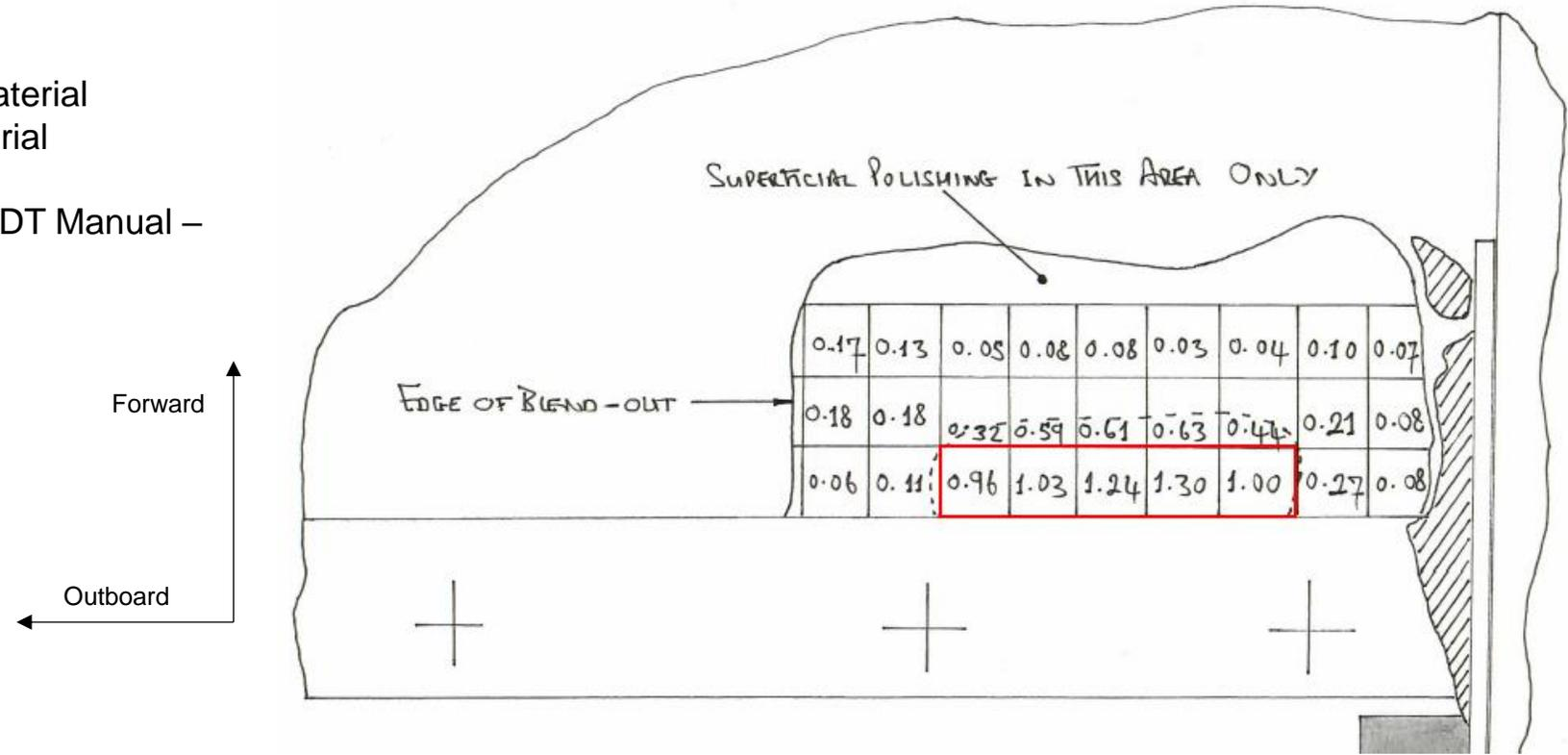
Depth Measurement performed with Digital Depth Micrometer
